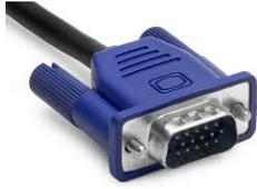
cable (found on the podium) to your computer. (The end of the VGA cable has an array of 15 pins in three rows in a trapezoidal rim, as seen on the left). If you have a MAC laptop, you MUST provide your own adapter cable to connect the VGA cable. It should look similar to the one pictured above right. If you want to use sound
