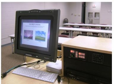
Computer: Small metal box (with a slit for a CD/DVD). Cables from the computer: USB cable (for a flash drive or other USB media), VGA cable (used to hook up your laptop), audio cable (used to hook up sound from your laptop).
